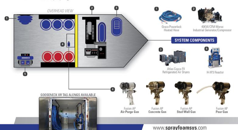
Setup in an 8x20 Cargo Hauler, the ProPAK XD4 can easily be towed by a 1 ton truck. There is plenty of room to carry up to three sets of foam and enough space to store ladders and scaffolding. The standard work bench stores all of your safety equipment.
