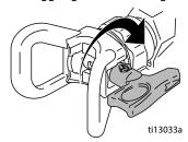
Engage trigger lock. Return Switch Tip to original position. Disengage trigger lock and continue spraying.
