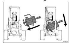
4 Swivel motor clamp. Tighten motor clamp and belt guard knob.
