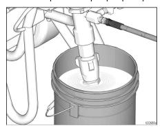
12. Trigger gun again into flushing fluid pail until paint appears.
