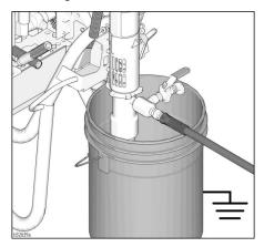
Turn prime valve to Drain position. Turn pressure control counterclockwise to lowest pressure.
