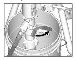
3. Set hydraulic pump valve OFF.
