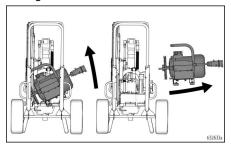
3 Tilt engine/motor. Install engine/motor. Install belt. Lower belt guard.
