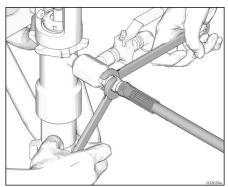
2. Install hose to spray gun and tighten securely.
