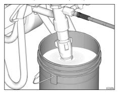
11. Trigger gun again into flushing fluid pail until paint appears.
