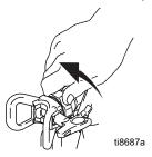
Remove displacement pump from paint and place in flushing fluid. Use water for water-based paint and mineral spirits for oil based paint.
