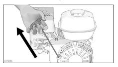
f. After engine starts, move choke to open.
