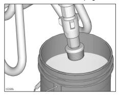
Unscrew and remove inlet strainer. Clean and replace strainer if necessary.
