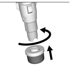
Fill throat packing nut with TSL to prevent premature packing wear. Do this each time you spray.
