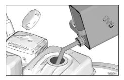
Check hydraulic oil level. Add only Graco Synthetic Hydraulic Oil, ISO Grade 46, 169236 (5 gallon/18.9 liter) or 207428 (1 gallon/3.8 liter). Hydraulic tank capacity is 1.25 gallon (4.75 liters).
