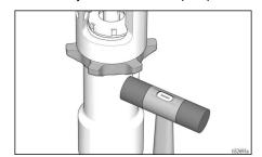
4. Push retaining ring up; push out pin.
