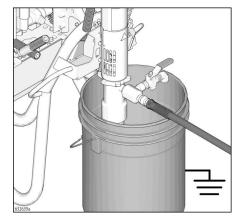
Turn prime valve to Drain position. Turn pressure control counterclockwise to lowest pressure.
