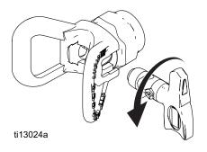
4. Screw assembly onto gun. Tighten.
