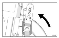
Increase pressure enough to start hydraulic motor stroking and allow fluid to circulate for 15 seconds; turn pressure down, turn prime valve to closed.
