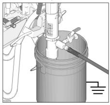
4. Turn motor switch ON or turn engine ON and start engine. Turn hydraulic
