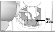
7. Check engine oil level. GASOLINE ENGINE
