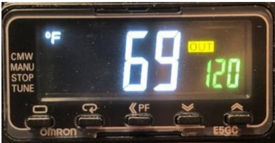
Figure 13: OMRON Temperature Controller
