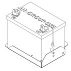
If you intend to use the unit's electric start system, you will need to purchase and install a battery to operate it. A 12 Volt battery, BCI group 26 rated at 500 CCA or larger is recommended for this electric start engine-generator set. Follow the battery manufacturers recommendations for servicing and charging prior to use. Connect the battery to the electric start system using the cables provided.
